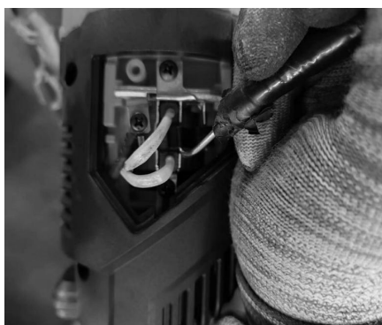
3.Pull Apart Coil Spring.
