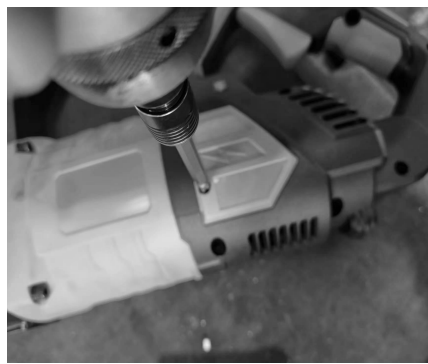
6.Cover the brush holder cover and turn the screws to secure the brush holder cover.
