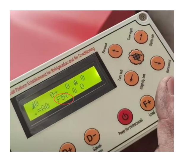
F57 Representing cruising speed control F+ ,F- (load+ , load - )
