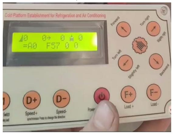
Press and hold the M key with your hand, then press the D+key (to start the machine)
