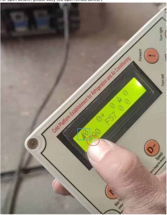
We start it  $1^{st}$  pressure M key then pressure D+ key , it will shown gear 3 and > symbol
