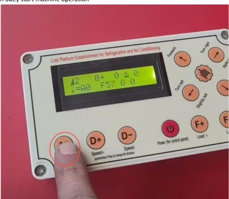
Press and hold the M key first ,then is D+ key
