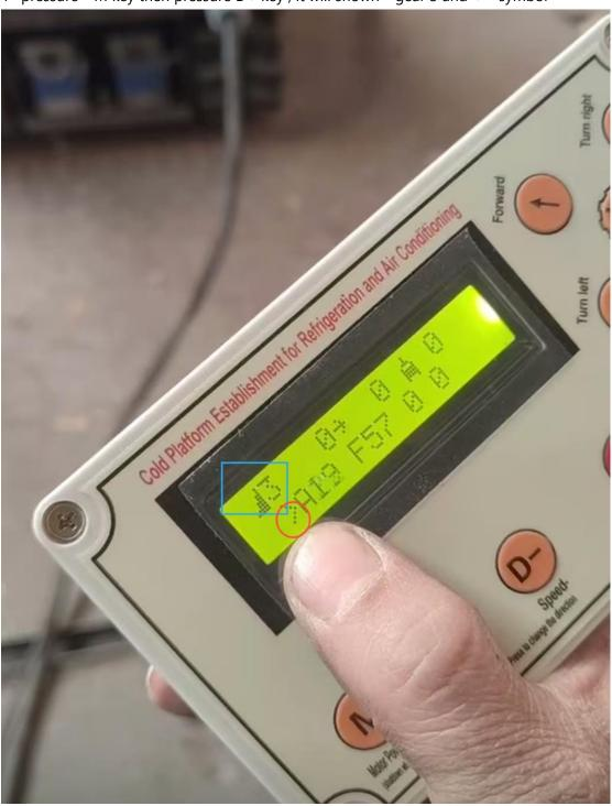
> symbol means machine start running, and it starts rotating in the positive direction.
