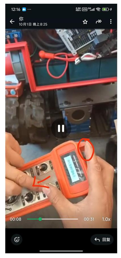
$5^{\text{th}}$  after done the step 4 press receiver side yellow light side button together longtime
